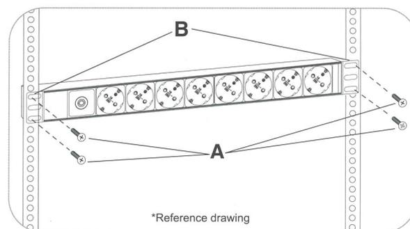
To mount the unit on rack, insert four screws from the package (A) through the unit's mounting ears (B) and into the rack's rails. Before installation, the user must ensure that the rackmount screws are suitable for holding the unit in the rack.
